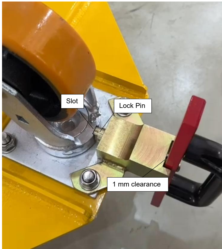
SWIVEL CASTER WHEEL LOCK MECHANISM Figure 6
