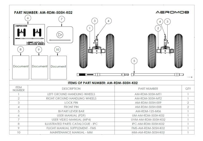
APPROVED USE: The HELIMOB 505H equipment has the function of suspending the aircraft from the ground and enabling the movement of the landed helicopter. The HELIMOB 505H is approved for use on Bell 505 models helicopters. The use of this equipment in other helicopter models or for functions not approved in the manual is expressly prohibited.
