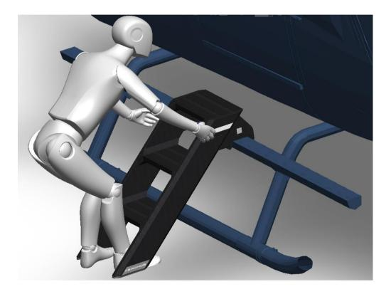
Embark or disembark along the ladder's specified path and avoid forcing the equipment in a lateral motion, perpendicular to the side rails, to ensure safety and avoid sliding.
